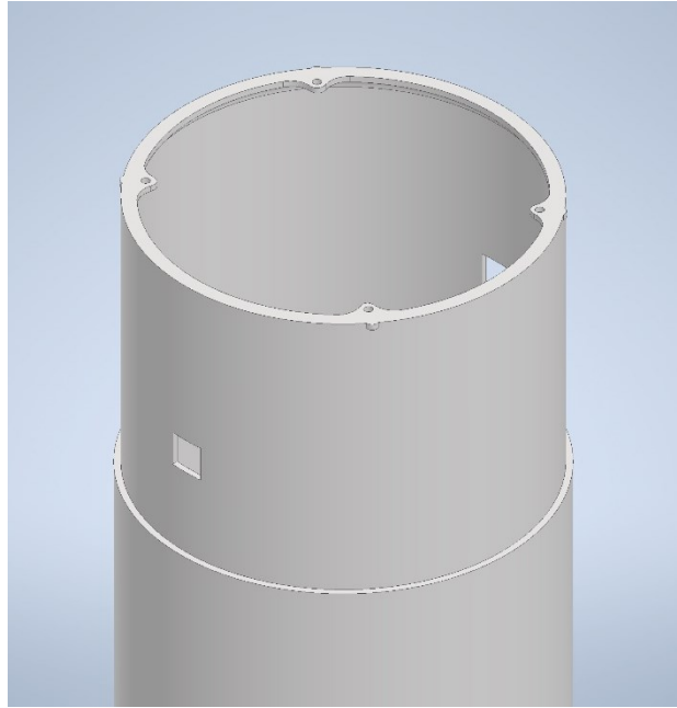
Figure 38: UpperTube with PCB Holder
