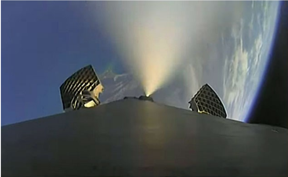
Figure 14: Falcon9 RCS during the Flip Maneuver [21]
