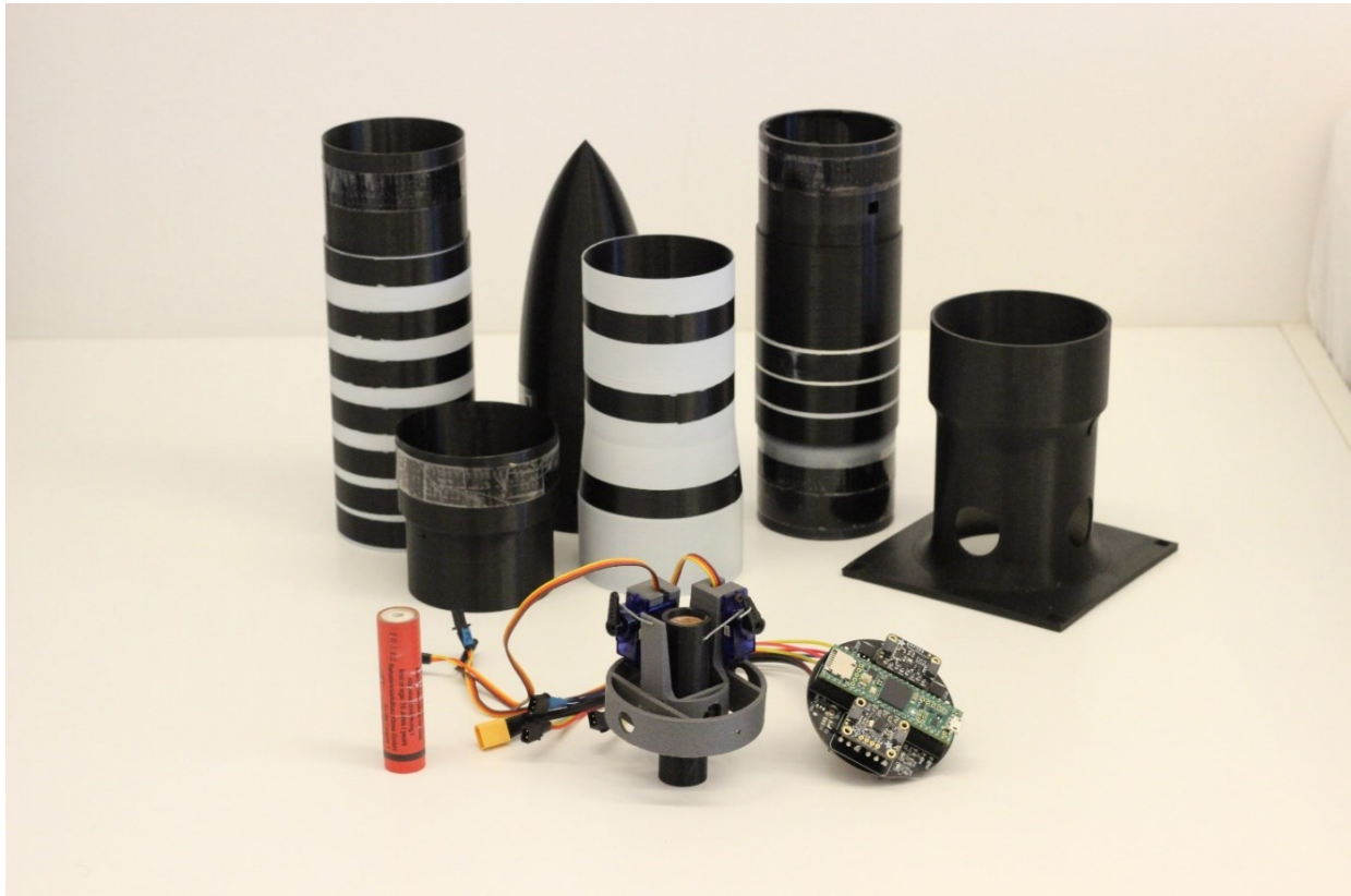
Figure 31: All Rocket Body Parts, TVC, D3-P Klima Rocket Motor and Flight Computer.
