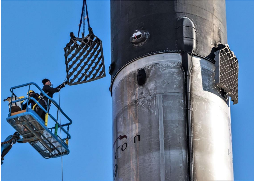
Figure 13: Grid Fins in Falcon9 Rocket [20]
