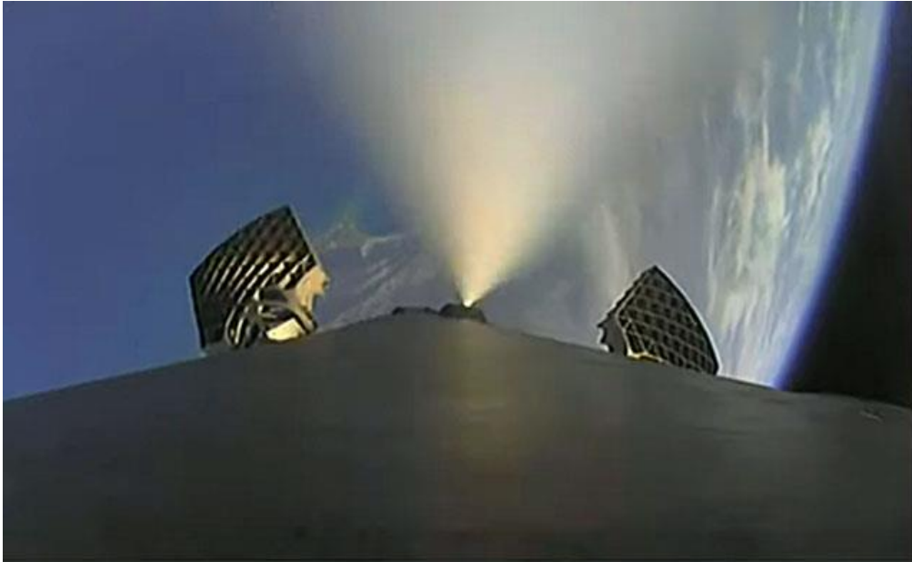
Figure 14: Falcon9 RCS during the Flip Maneuver [21]
