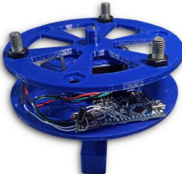
Figure 15: Fully Assembled Reaction Wheel [22]
