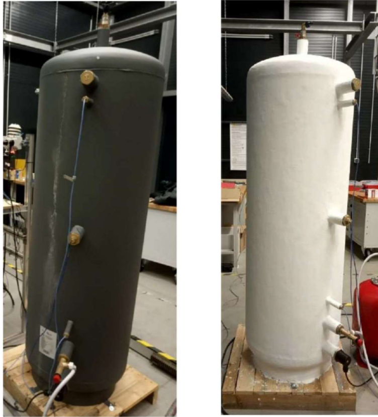
Fig. 2: Measurements of a heat storage tank without thermal insulation (left) and a heat storage tank with thermal insulation coating (right) under conditions of free air convection, Source: UCEEB
