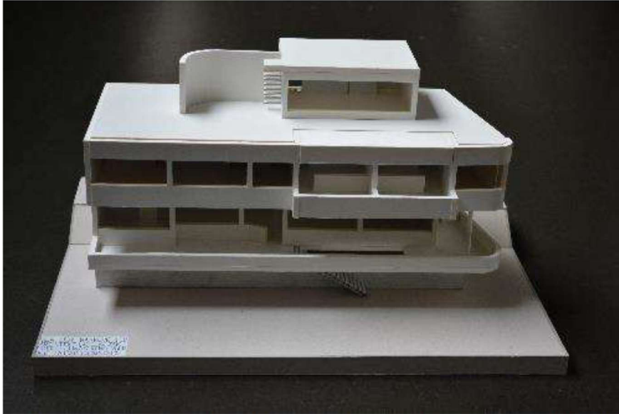
Fig. 4 – Architectural model of residential building is ready for measuring and for adjusting the reflectivity of internal surfaces, reflectivity of outdoor terrain and various window glazing.
