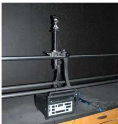
Fig. 3 – Sensor of illuminance meter Precision Photometer Bruel-Kjaer 1105 on photometric desk
