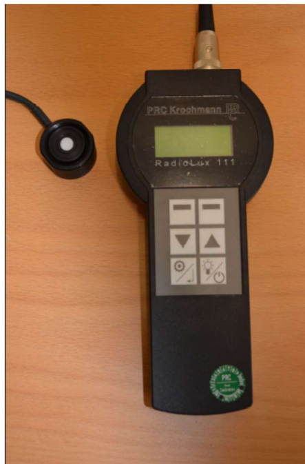
Fig. 3 – Testing illuminance meters PRC Krochmann – RadioLux 111
