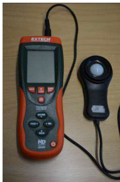
Fig. 2 – Testing illuminance meters Extech HD 450
