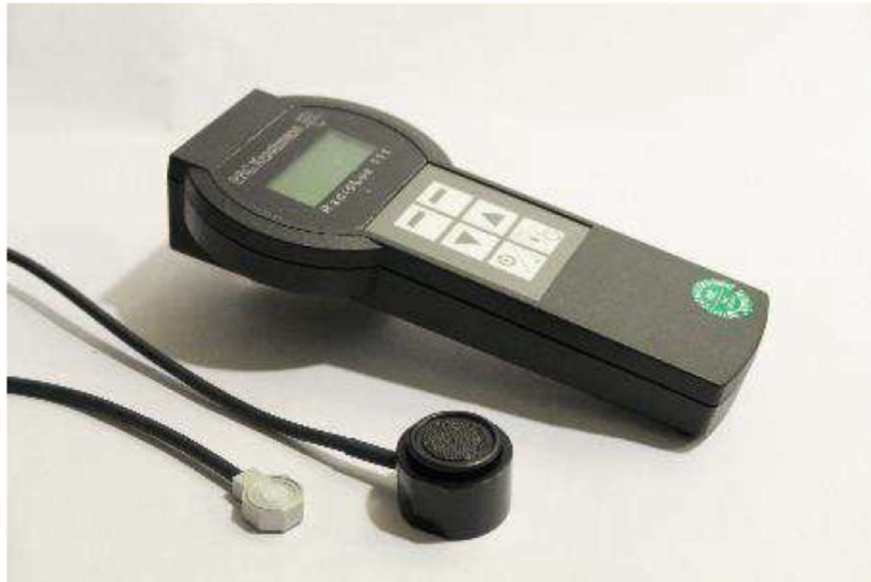
Fig. 1 – Illuminance meter RadioLux 111 with photometric heads – first is for common measurement and second for measurement in models
