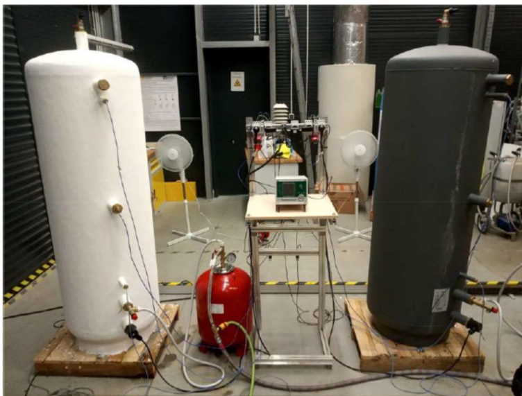
Fig. 3: Additional heat loss measurements of heat storage tanks with and without thermal insulation with added fans, Source: UCEEB
