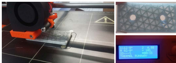
Fig. 2.3 Third test print of 100% b-PET under configuration B - unfinished
