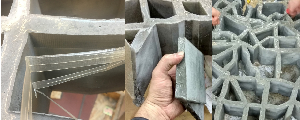
Fig. 6.3 structure mould- ed with recycled filament moulds
