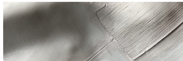
Fig. 7.4 Perpendicular stripe patterns caused by the technology principles.
