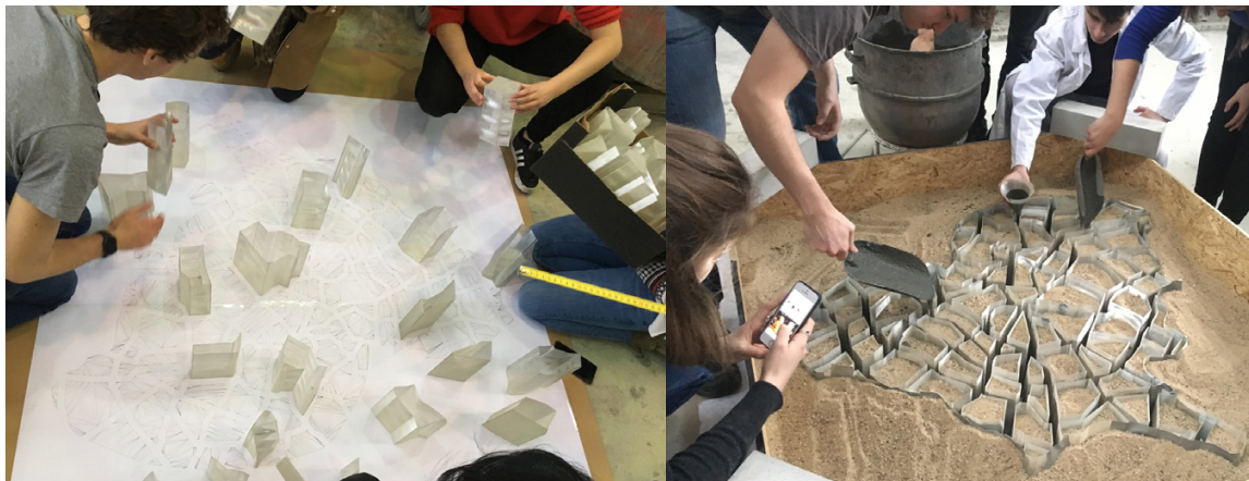
Fig. 6.4 3D printed moulds distribution and filling with sand
