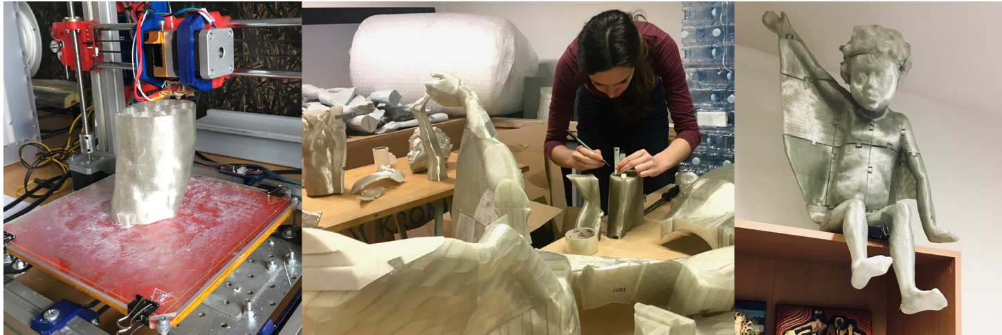
Fig 7.3 From 3D printing pieces to ready statue
