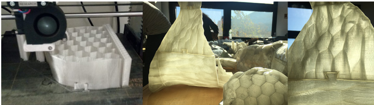
Fig. 7.5 the influence of infill on the weight and design of the pieces.
