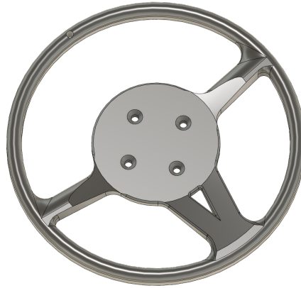
(b) : 3-D model of steering wheel
