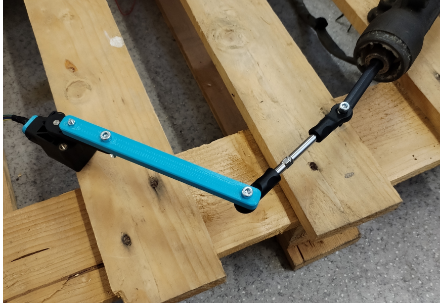
Figure 5.5: Connection of angle sensor on the PSU
