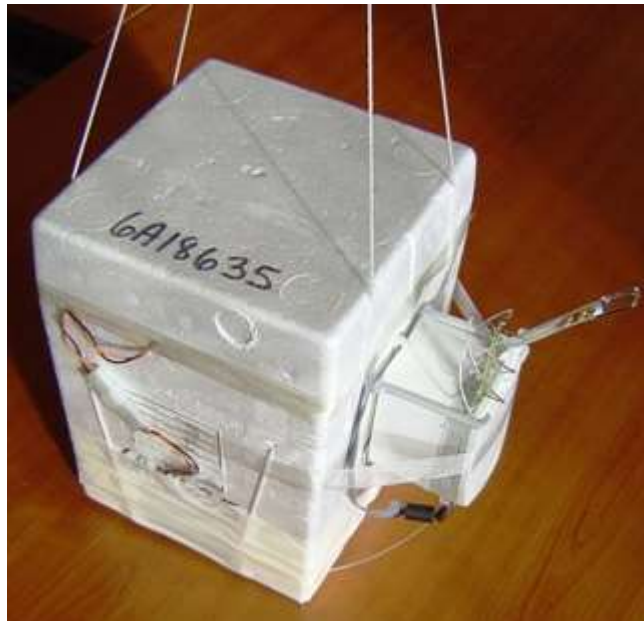
Image 17 Box with ozone sensor and radiosonde (on side)
