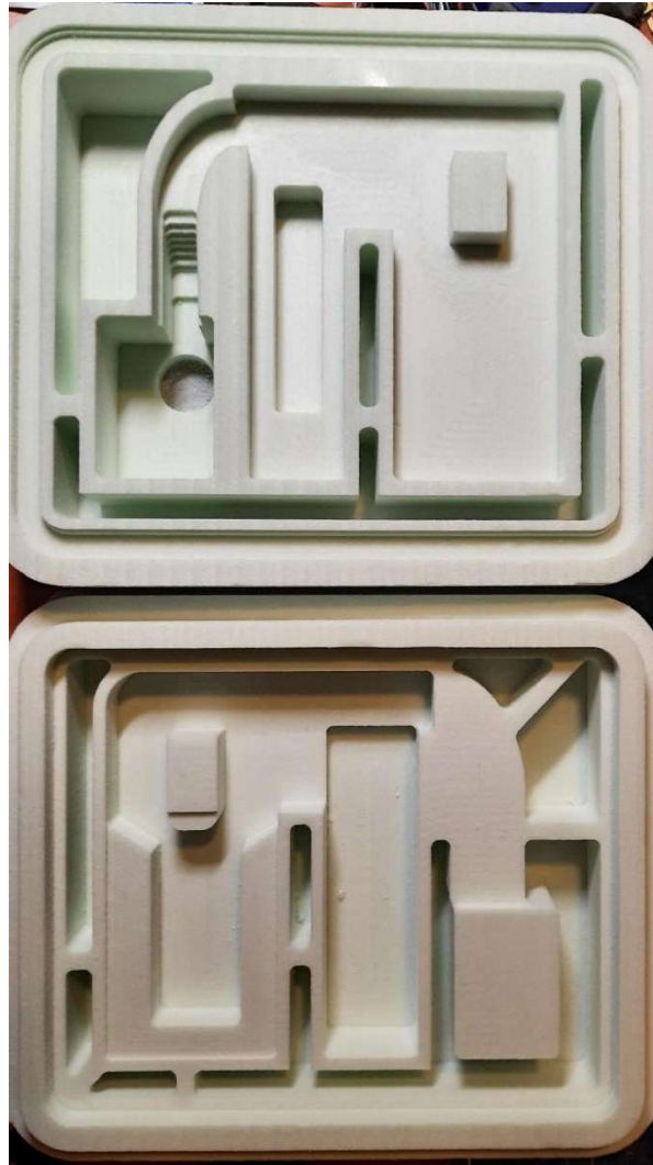
Image 18 StratoSat's outer protective casing made of Extruded polystyrene Source: Tomáš Lapeš (2023)
