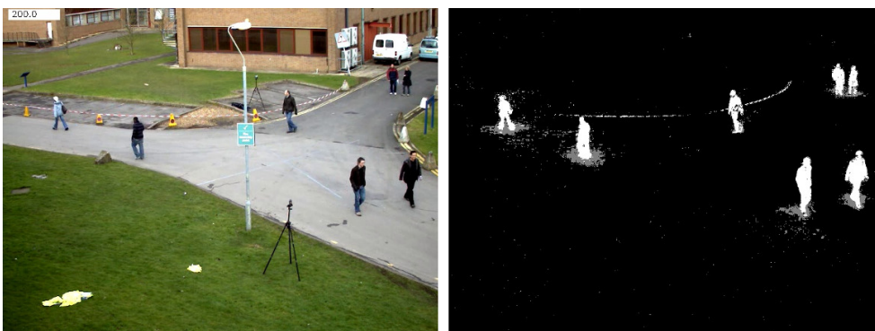
Figure 4.16: Example of the MOG2 background subtraction algorithm from the OpenCV library [91].
