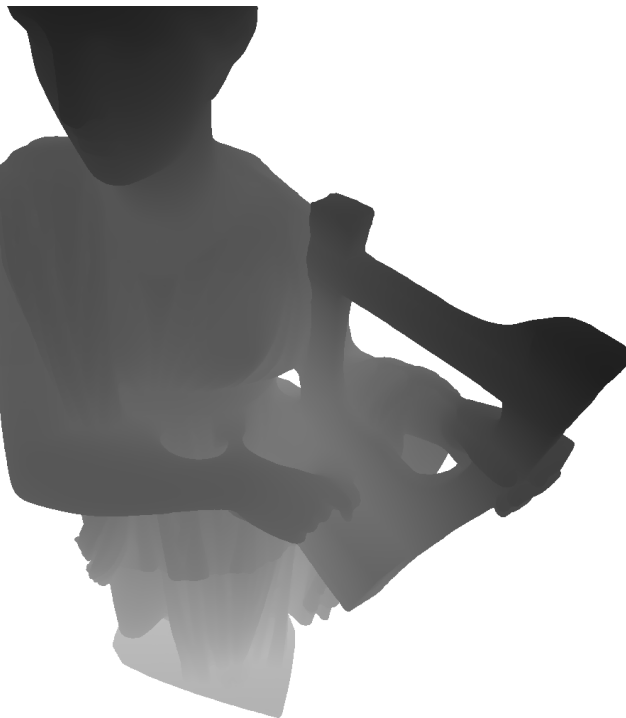
Figure 5.18. Each pixel of erato mesh is assigned a grayscale color based on the distance from the camera, with darker pixels being closer.
