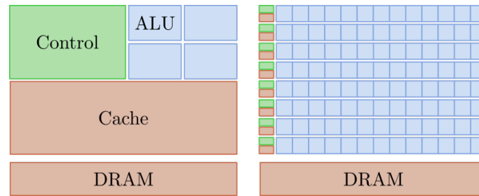
Figure 2.3. Difference between CPU and GPU architecture design. A huge portion of the die area of the CPU on the left is filled with cache hierarchy and control unit to achieve low latencies. The GPU on the right is filled mostly with the computation cores [8].
