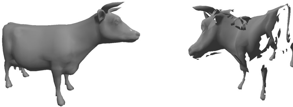
Figure 5.9. When disabling back-face culling with a shortcut, keeping the culled triangles culled until enabled again, the rotation of the camera on the right reveals which part of the cow object was back-face culled when viewing from the angle on the left.
