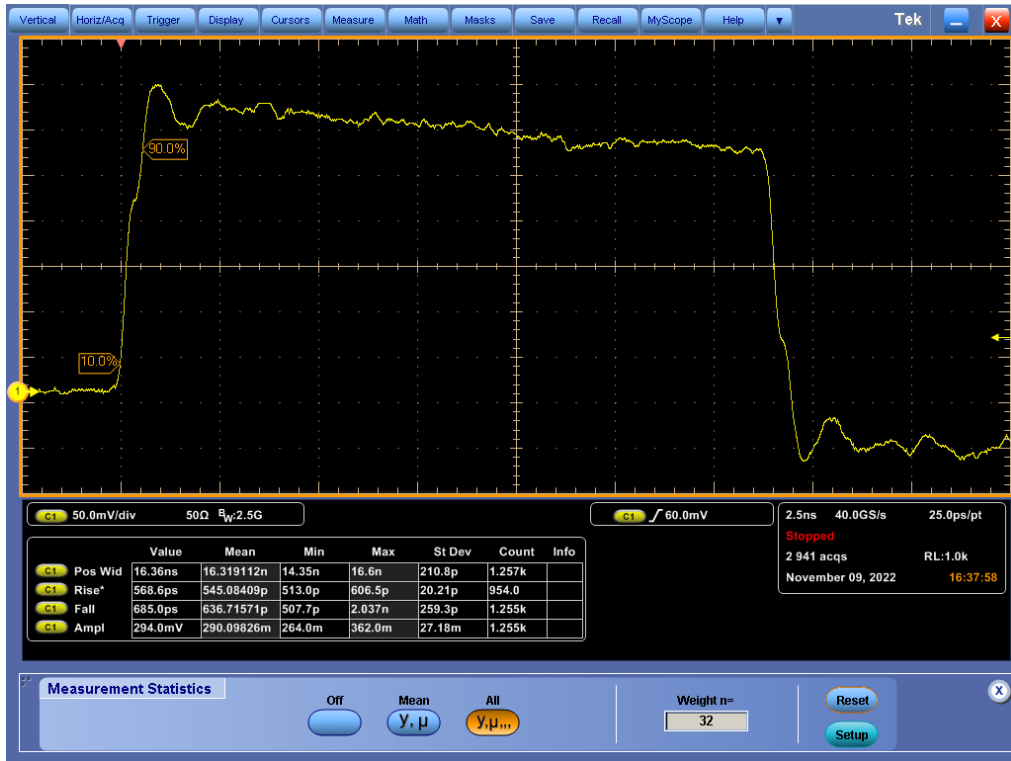
Figure 29. Oscilloscope screenshot showing the output pulse of the single photon detector, an overshoot is visible on the rising and falling edge.
