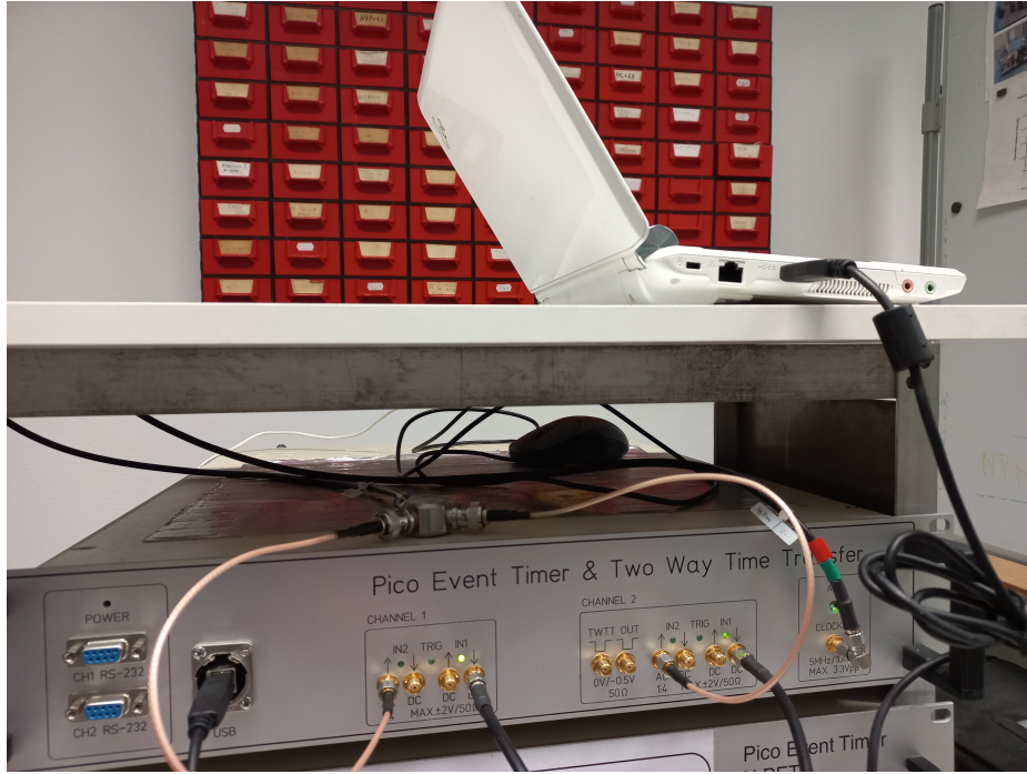
Figure 26. Photo of the time measurement system, consisting of the NPET clock and computer, that was used for confirming properties of the new single photon detector featuring the ADCMP573 comparator.
