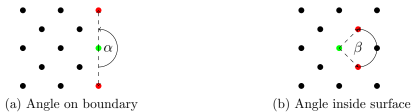
Figure 3.4: For green point, \mathbf{p} and red points \mathbf{q}_1, \mathbf{q}_2 \in N_{\mathbf{p}} , angle \alpha between boundary points is much bigger (a) than angle \beta constricted by two interior points (b).
