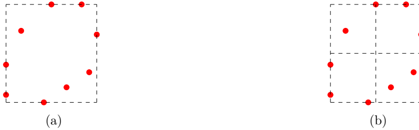
Figure 4.4: Boundary points with surrounding rectangle too big for accurate scanning (a) and the same rectangle after division to appropriate smaller areas (b).
