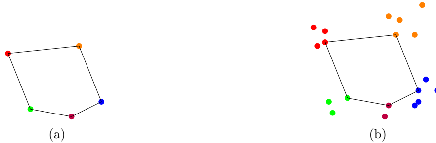
Figure 4.8: The illustration of the solution of TSP task (a) and the GTSP task (b). The points with the same color belongs to the same cluster.
