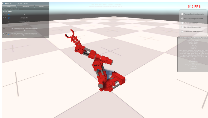
■ Figure 5.10 RR1 simulation prototype in Unity
