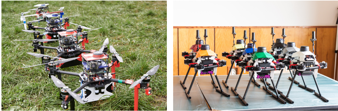
Figure 4.3: Different types of UAVs built from the MRS Modular UAV Hardware Platform.
