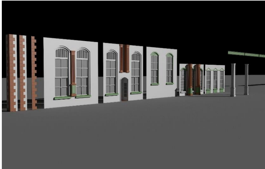
Figure 3.4: Example of modular components [Tho]
