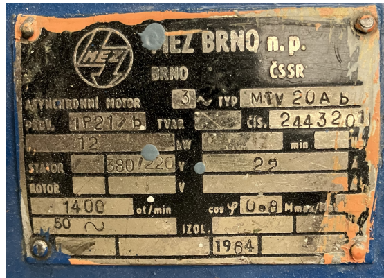
Figure 4.2: Induction motor rating plate
