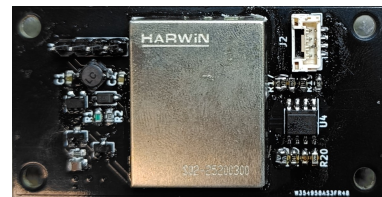
Figure 2.17: The back side of PCB with shielding box
