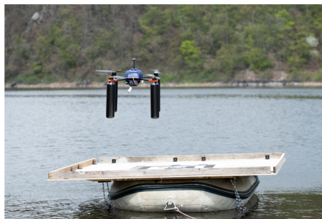
Figure 1.3: Illustration of an autonomous UAV landing on an oscillating platform as presented in [1].
