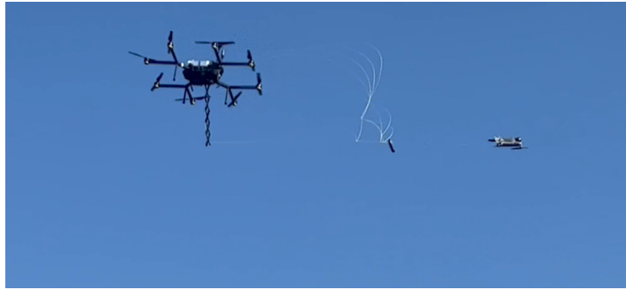
Figure 3.24: Photo of the successful interception attempt by Eagle One catching DJI Mavic
