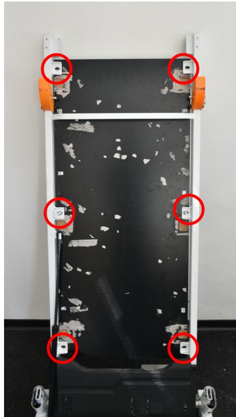
Figure 3.1: Position of strain gauges on the treadmill
