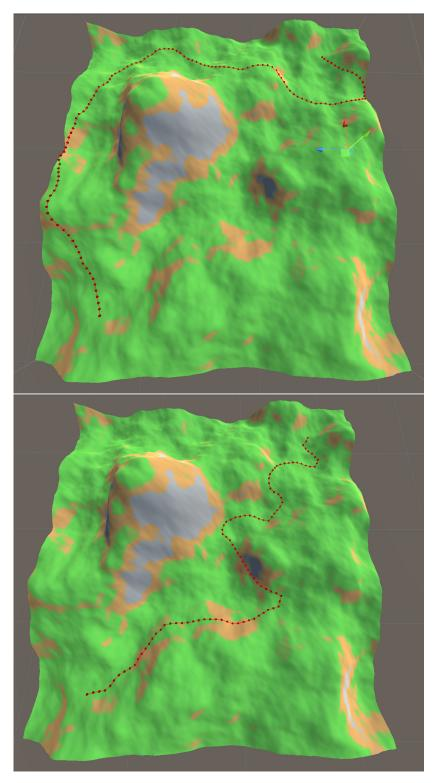
**Figure 3.9:** Two different winding paths generated using local path-finding. The first one had default weights. The second one had the Direction To Goal weight lowered to create a less straightforward path.
