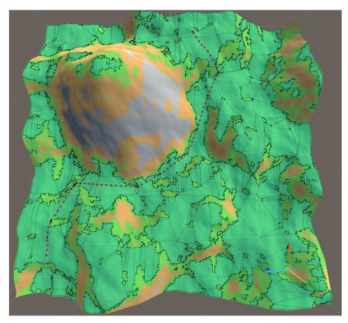
**Figure 3.8:** A straightforward path generated using global path-finding with a NavMesh (turquoise areas). Additionally, for better visibility, the corner points have been connected by more points using linear interpolation.
