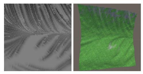
**Figure 3.2:** The left image is a hydraulic erosion texture of a chunk, where gray means no change in height, darker color means the terrain is subtracted, and lighter color means the terrain is heightened. The right image is the texture applied on a chunk.
