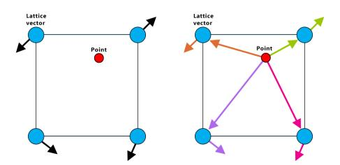
**Figure 2.2:** Algorithm described by subsection 2.1.3. The first picture shows the base setup with lattice vectors and the point at which we want to generate the height. The second picture shows the pairs of vectors that are used for the dot product.
