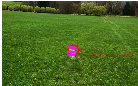
Figure 6.11: Processed image of the color camera when detecting radiation source positions with marked possible threatening object obtained by measurement in real environment test.
