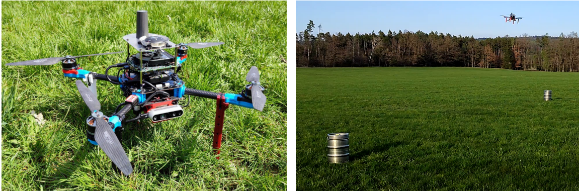
(a) The UAV model used in a real experiment with all sensors and components based on the Holybro X500. (b) Example of the environment in which the real experiment was performed with two radiation sources and one flying UAV.
