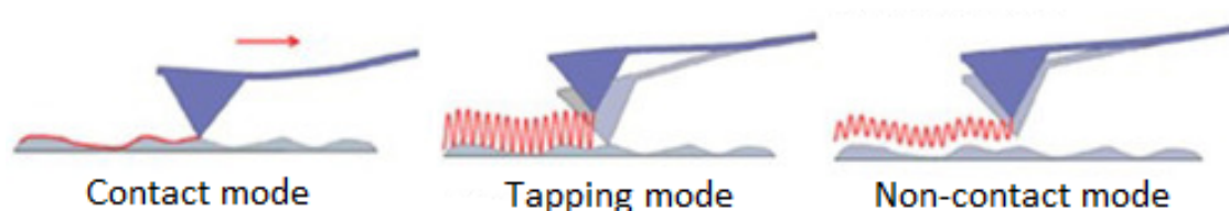
Figure 1.3: Graphical representation of different types of imaging modes used to obtain AFM images. Taken from JPK Instruments handbook and modified. [9]
