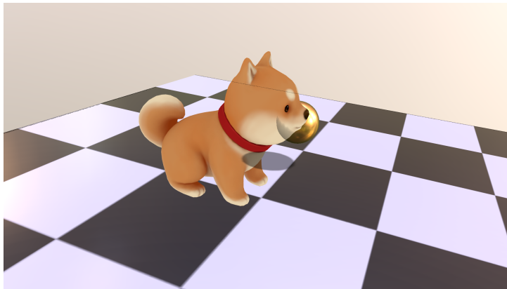
Figure 3.5: Loaded glTF model of a dog causes errors in shadow rendering. Behind the model is an X3D defined sphere above ground, casting a shadow that can be seen through the glTF dog model. The glTF model itself does not cast shadows.
