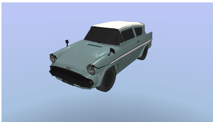
Figure 3.10: Usage of PBR textures shown on an X3D model with X_ite library. Note that the environment mapping and image based lighting is not yet implemented.
