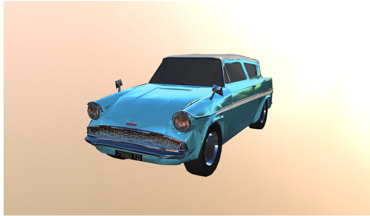
Figure 6.2: Car low-resolution X3D model with PBR textures shown in the new Simulink 3D Animation viewer.
