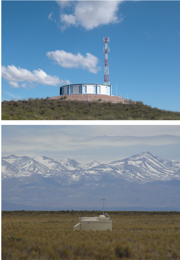
Figure 3.4: Los Leones fluorescence detector enclosure (top) and surface detector station (bottom) (4).
