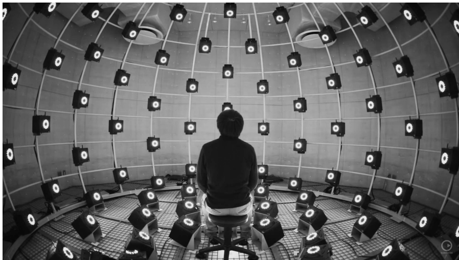
Figure: Anechoic chamber for surround sound - for the purposes of this thesis author created the virtual space for Surroundsound in PureData and Unreal Engine, see Appendix A on authors GitHub
