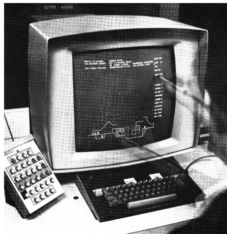
Figure: URBAN 5's overlay and the IBM 2250 model 1 cathode ray-tube used for URBAN 5 (source: openarchitectures.com )
