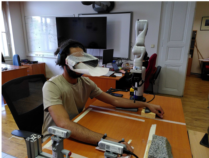
Figure 3.3: The first pilot experiment setup, where the robot slides over the participant's left arm according to the movements of the right arm. There are three Qualisys markers on the right arm, two on the robot, and four on the calibration triangle.
