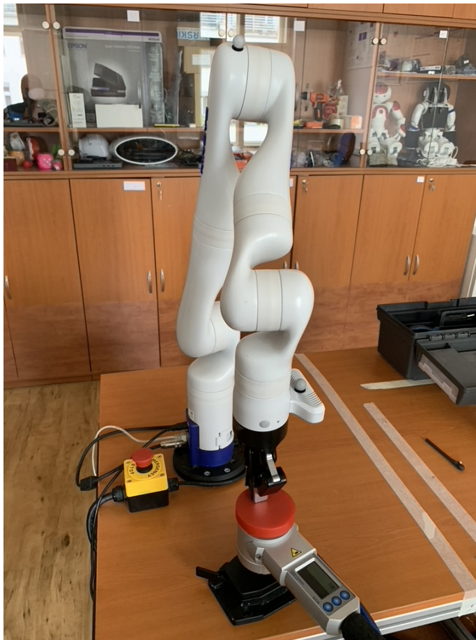
Figure 4.7: Passive robot falling onto the measuring device from the top.
