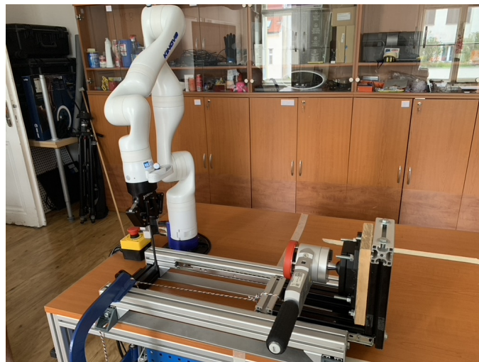
Figure 4.10: Setup for measuring the forces in the direction of the participant. Device was hit by the metallic end-effector.
