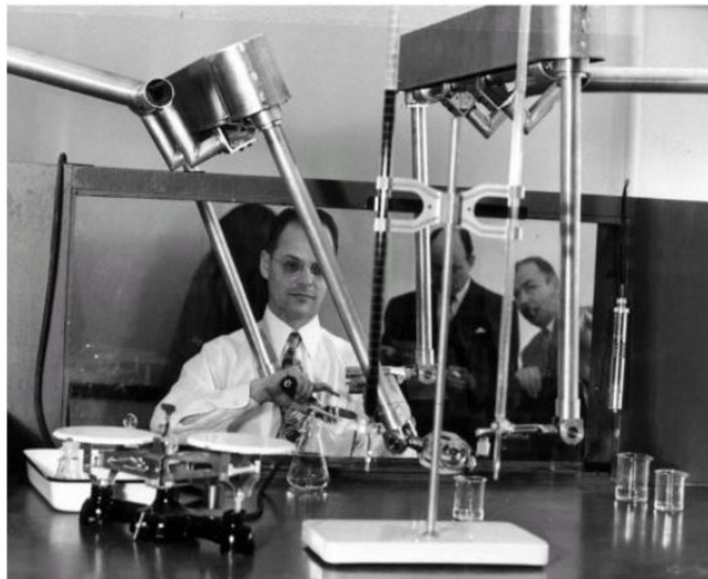
Figure 2.2: The first modern master-slave pantograph made by Goertz at Argonne National Laboratory, from [9].
