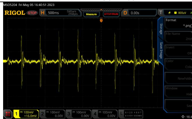
c – 2 Hz data with a 1 MΩ load measured with RIGOL MSO5204, d – 2 Hz data with a 19.6 kΩ load measured with RIGOL MSO5204.
