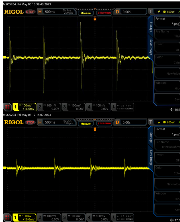
a – 1 Hz data with a 1 MΩ load measured with RIGOL MSO5204, b – 1 Hz data with a 100 kΩ load measured with RIGOL MSO5204.
