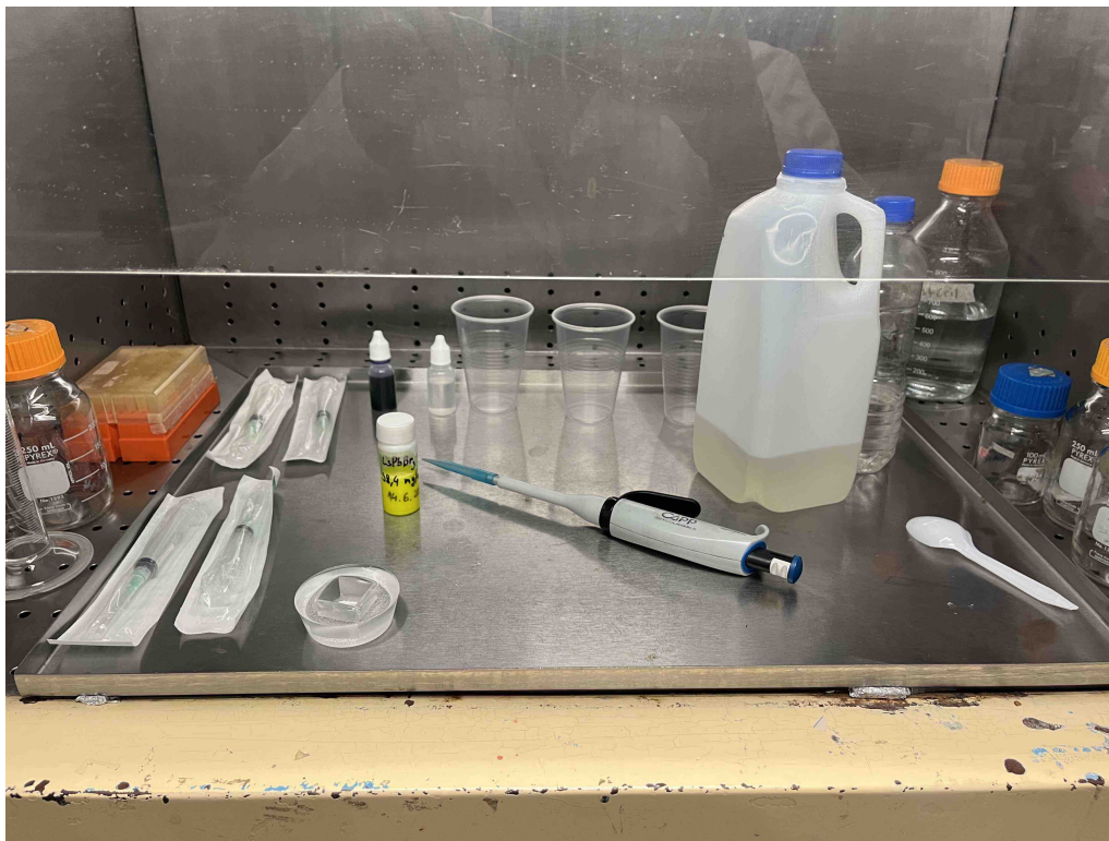
Figure 3.6: Set-up used for the production of the styrene composites with \text{CsPbBr}_3 nanocrystals. Used materials: epoxy resin (white jug with blue cap), styrene (white bottle with blue cap), toluene solution with \text{CsPbBr}_3 nanocrystals (yellow vial), MEKP (transparent vial), and RP-128 (violet vial). Used tools: disposable syringes, plastic cups, plastic spoons, pipette, and silicone mould.
