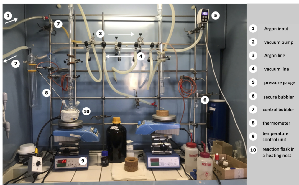
Figure 3.1: Photograph of the Schlenk line used for the synthesis of \text{CsPbBr}_3 nanocrystals. Figure taken from Ref. [37].
