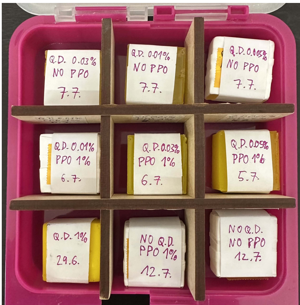
Figure 3.14: Box containing the produced \text{CsPbBr}_3 nanocomposites in silicone matrix for their easy classification, transport, and storage. Each sample is labelled with the concentration of the added compounds to the base according to the final weight and with the date of production of the sample during the year 2022.
