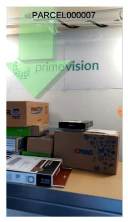
FIGURE 2. Highlighting in AR the location of the parcel to be delivered next.
