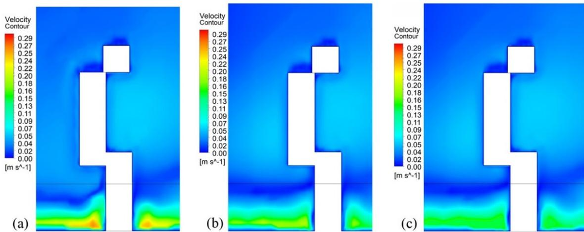
FIGURE 5. Simulated velocity contours around a human model at three distances from the radiant panel, namely distance of human model from panel, namely 20 cm (a), 35 cm (b), and 55 cm (c).
