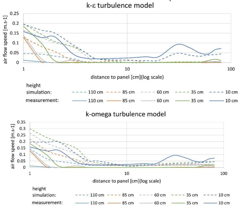
FIGURE 3. Velocity as a function of distance from the panel for two different turbulence models.
