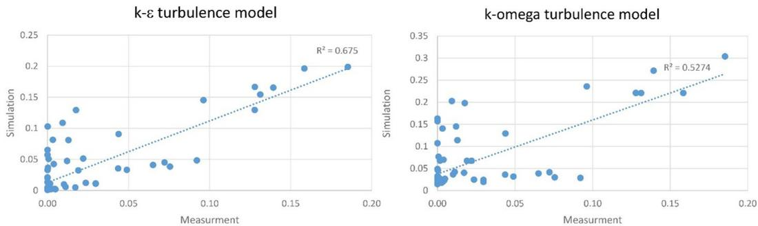
FIGURE 4. Simulated velocities plotted against corresponding measurements for two different turbulence models.
