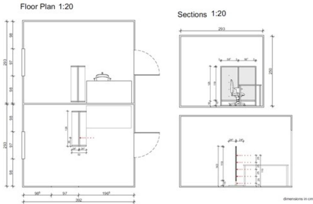
FIGURE 2. Floor plan and sensors locations at the test room.
