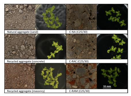
FIGURE 3. Example of *Lemna minor* semichronic toxicity test performed with 80 % leachates of natural and recycled aggregates fraction 0-4 mm (left) and 80 % leachates of concrete mixes (C25/30) based on the relevant aggregates (right). C-NA – reference concrete, C-RAC – concrete containing concrete-derived recycled aggregate, C-RAM – concrete containing masonry-derived recycled aggregate.
