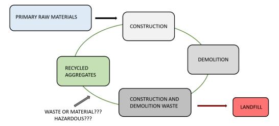
FIGURE 1. Life cycle and recycling possibilities of primary raw materials.
