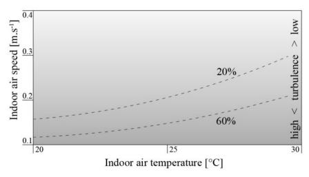
FIGURE 3. Illustrative exemplification of standard-based specification of an IEQ indicator (maximum permissible air flow speed) and its value as a function of indoor air temperature and turbulence intensity (based on standards DIN EN 15251 and DIN EN ISO 7730).
