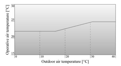
FIGURE 2. Example of a standard-based IEQ indicator (operative air temperature) and its value as a function of the outdoor air temperature (based on standards DIN EN 15251 and DIN EN ISO 7730).
