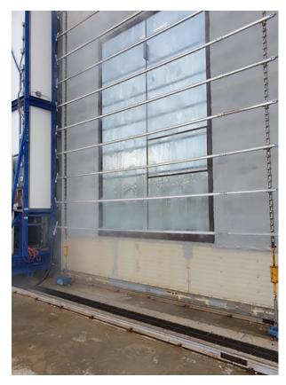
FIGURE 3. Watertightness performance under static pressure on mock-up 01.
