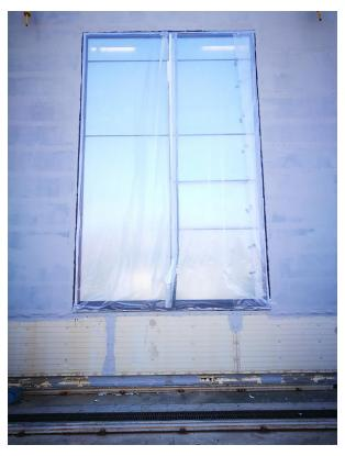
FIGURE 1. Air permeability test on mock-up 01.
