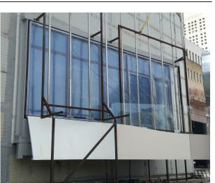
FIGURE 2. Air permeability test on mock-up 02.
