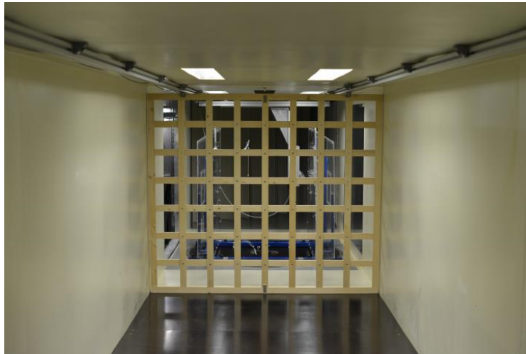
Figure 5.3: Vortex generating grid to create turbulent flow in the range of 5 to 30%.
