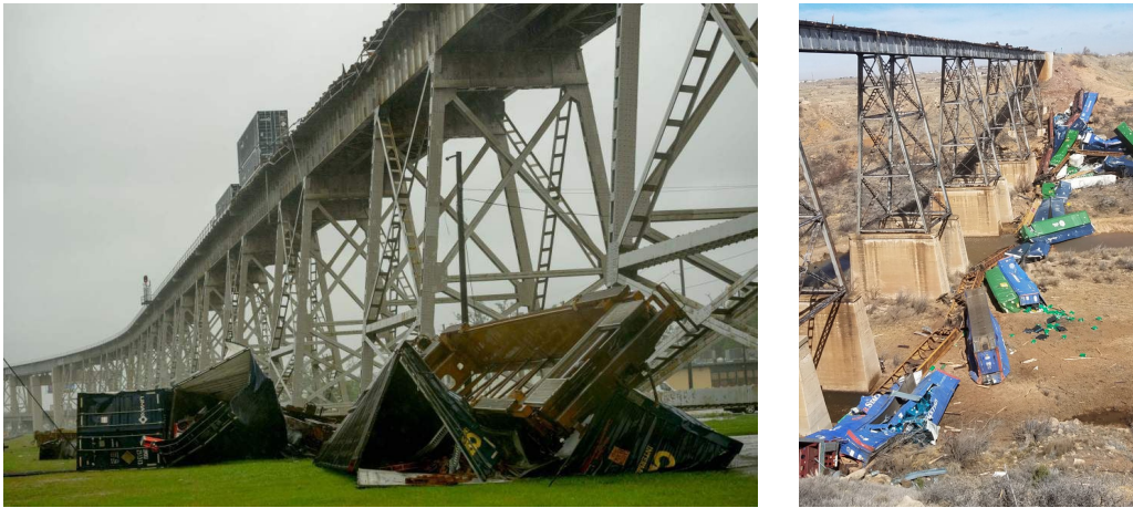
Figure 2.2: Wind induced train derailment of train passing a bridge, Huey P. Long Bridge Louisiana US (left), bridge over Canadian river New Mexico (right).
