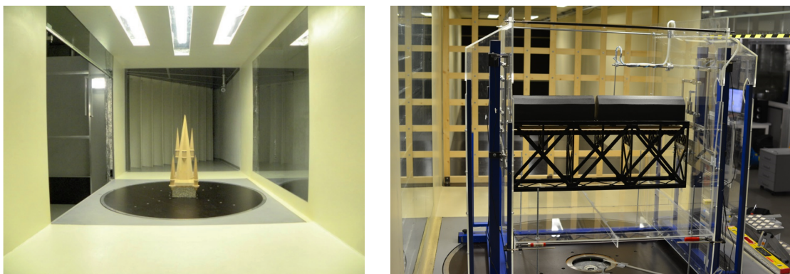
Figure 2.5: Structural models in the wind tunnel, climatic section (left) (Kuznetsov et al., 2015), aerodynamic section (right) (Ryjacek et al., 2017).
