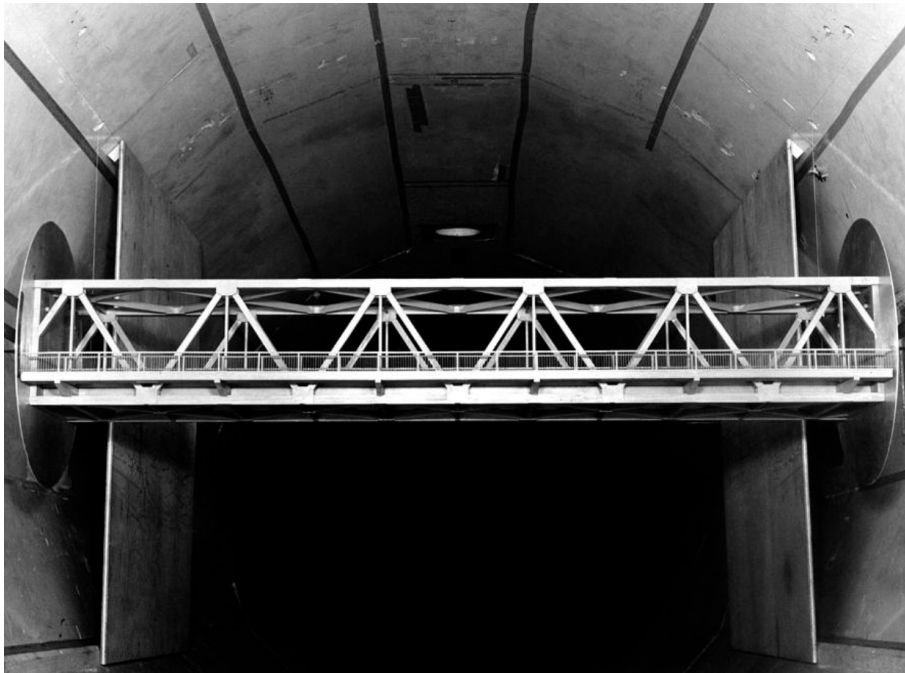
Figure 2.3: Wind tunnel test of truss girder bridge sectional model (NPL, 1954).
