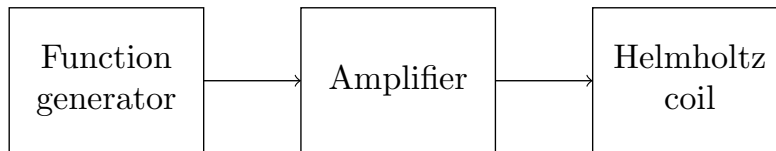
Figure 3.3: Gaussmeter calibration scheme
