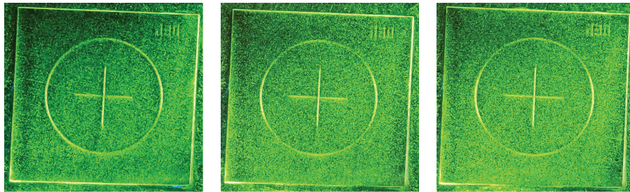
(a) classical multidirectional magnetization: two current sources (b) time-multiplexing: two current sources (c) time-multiplexing: one current source
