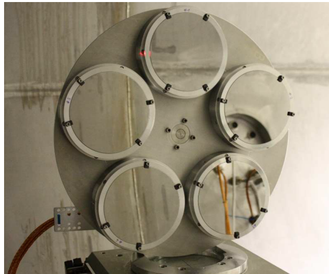
Fig. 7.2: The five mirror samples mounted in the sample wheel holder. Image from inside the PANTER chamber, the wheel stands on manipulator.
