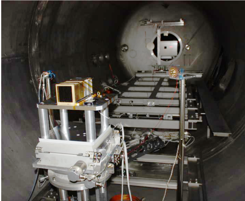
Fig. 9.14: HORUS II in vacuum chamber. On the right at the beginning of the vacuum tunnel can be seen the mask, closer the QCM on its mount.
