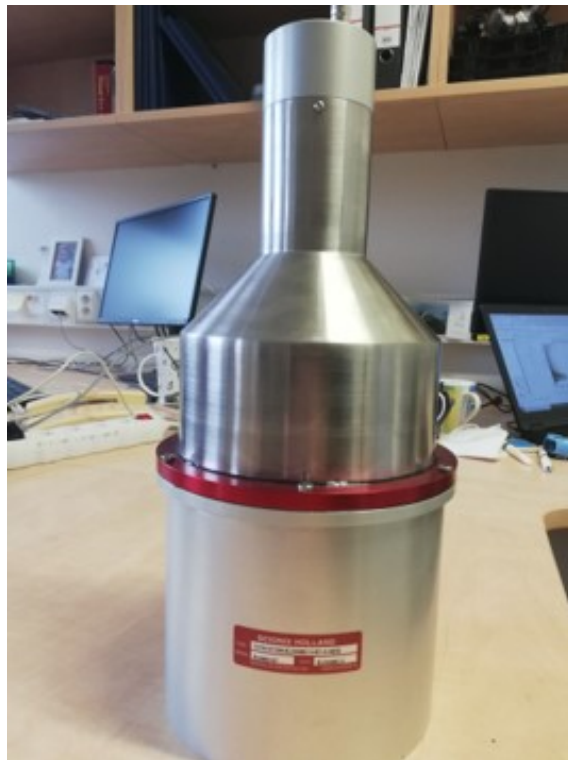
Figure 6.2: The large 5x5" scintillator EJ-309B2.5 coupled with photomultiplier tube 9390B.
