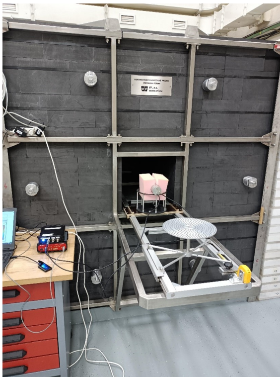
Figure 6.18: A photograph of irradiation of 2x2" scintillator at a prism made of carbon at Czech Metrological Institute. Six AmBe neutron sources are inserted inside the prism.
