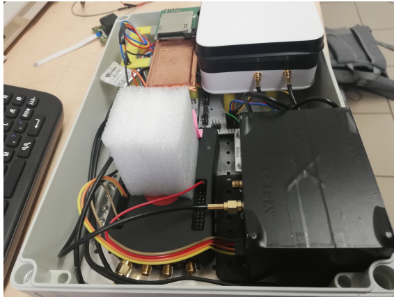
Figure 4.24: A photograph of the Airwatch system that is used for the measurements onboard aircraft. The Airwatch contains a detector based on plastic scintillator, Si based detector AIRDOS and NaI(Tl) scintillator.
