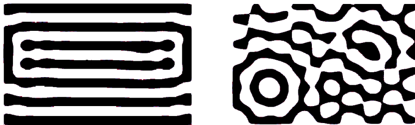
Figure 1.2: Pattern in a system with Schnackenberg reaction and without unilateral regulations on the left, with unilateral regulations on the right. Both systems had the same diffusion parameters and Neumann b.c.
