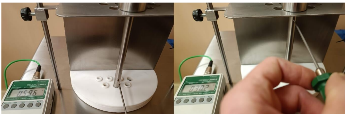
Figure 44: Surface temperature measurement, temperature in bath is 220\text{ }^{\circ}\text{C} nominal
