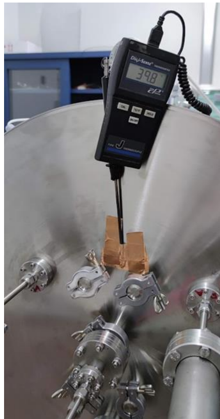
Figure 70: Surface thermometer attached to the flange of the furnace
