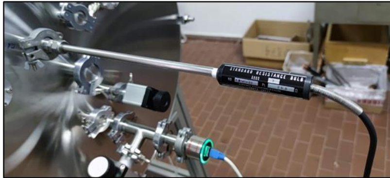
Figure 69: SPRT inserted in a thermometry well that is sealed across the head flange of the furnace.
