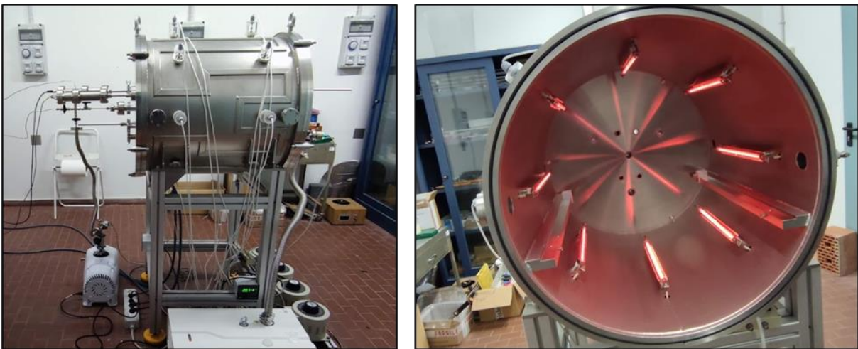
Figure 60: Heating furnace used in HTAGT research, placed on a framed supporting structure.
