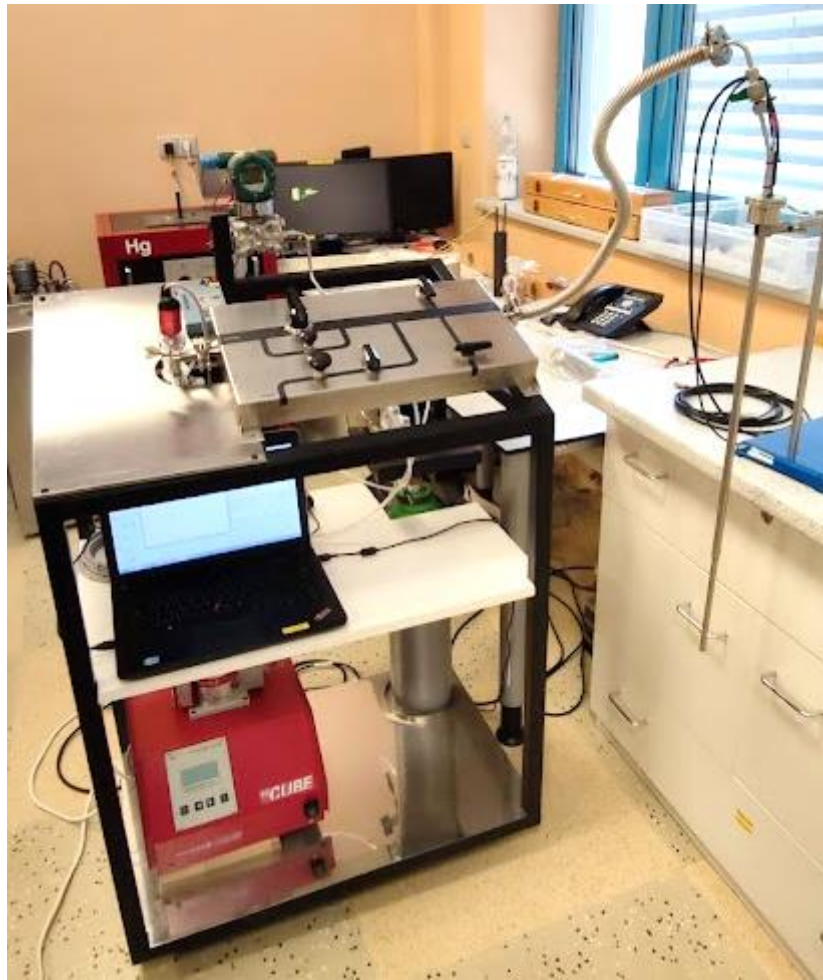
Figure 40: The mobile gas management system connected to PAT
