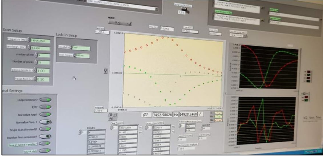
Figure 11: Example of LabView application, fitting the quadratic function to acoustic resonance mode
