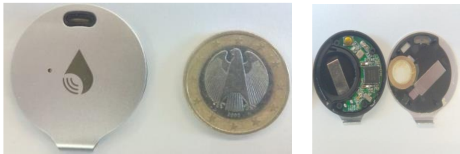
Figure 40. Tracking device used for the purpose of material decomposition using multi-bin X-ray tomography.
