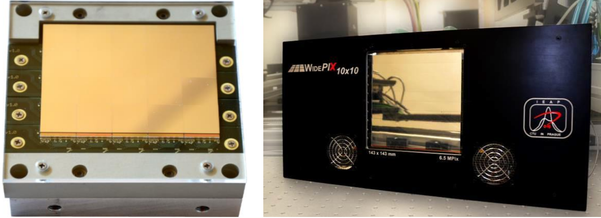
Figure 21: Left) WidePIX 4 \times 5 detector of 20 tiles of edgeless Timepix detectors. Right) WidePIX 10 \times 10 detector composed of 100 edgeless Timepix chips.
