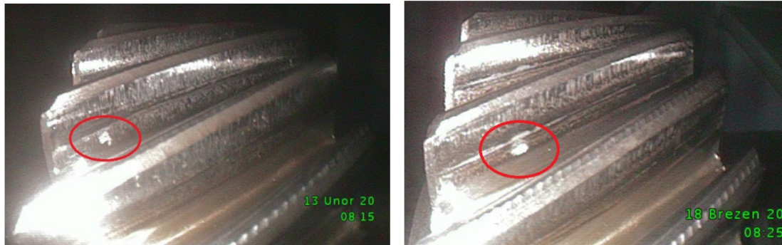
Figure 7-5: Pitting on PM HIP:ed gearwheel (6 th speed) – gearset 1 - after 85 hours (left), gearset 2 – after 41 hours (right).
