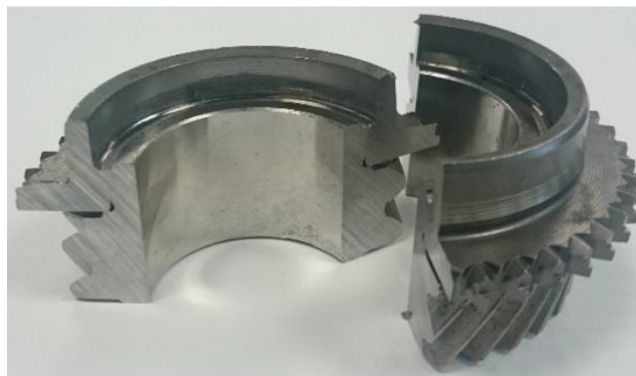
Figure 7-7: Section for checking the weld quality between the synchronizing and PM gearwheel (3 rd speed)
