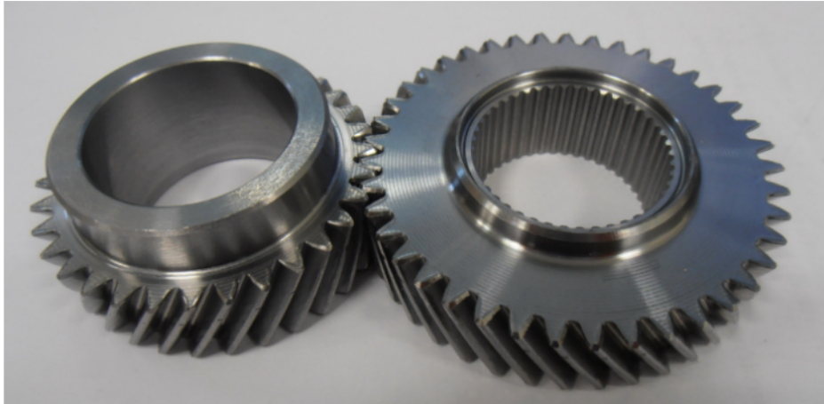
Figure 7-3: Turned basic gear shape with milled gearing and machined splines (3 rd speed).
