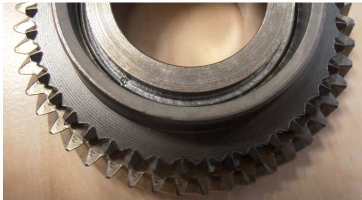
Figure 7-6: Welded synchronizing to a gearwheel (6 th speed).
