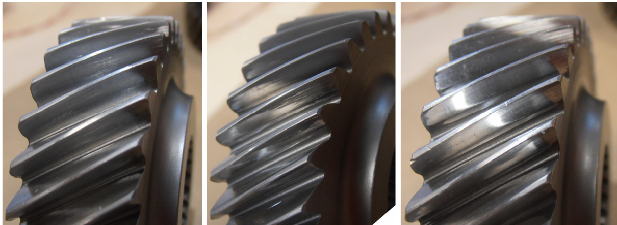
Figure 7-41: Small gear ( z=31 ) after coast flank grinding. Gear's part not ground (left), partly ground (middle) and fully ground (right).
