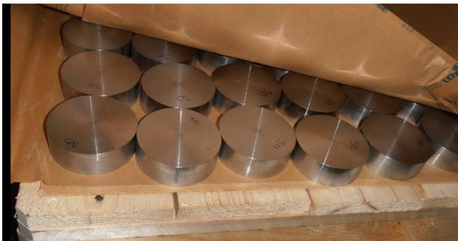
Figure 7-2: Semi-finished blanks – sintered, HIP:ed and turned PM pucks.
