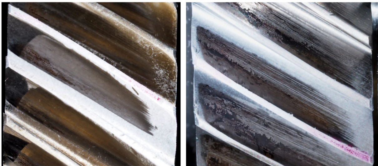
Figure 7-44: Result of summative contact pattern test of asymmetric rolled gearset after coast flank grinding – large gear ( z=48 , left), small gear ( z=31 , right)
