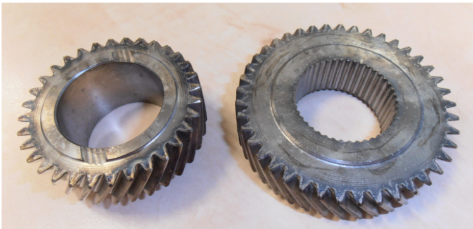
Figure 7-4: Gearset of the 3rd speed after the heat treatment.
