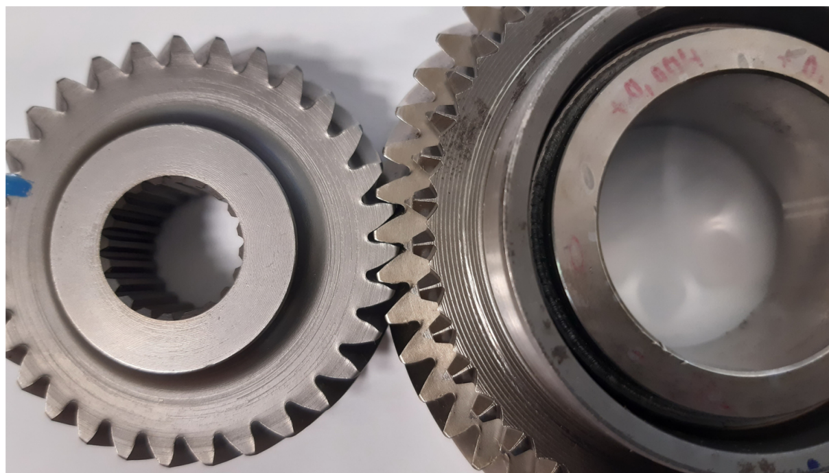
Figure 7-37: Asymmetric rolled PM gearset of the 6 th speed ready for testing
