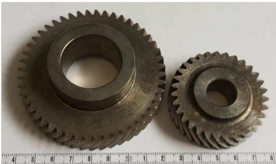
Figure 7-26: Asymmetric rolled PM gearset of the 6 th speed ready for material properties investigation
