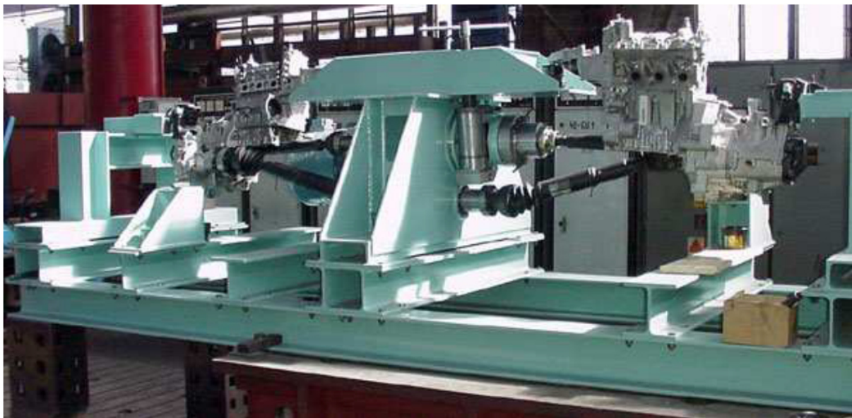
Figure 5-1: Back-to-back test rig for endurance tests of the gearbox MQ200 designed at TU of Ostrava – original appearance [21].
