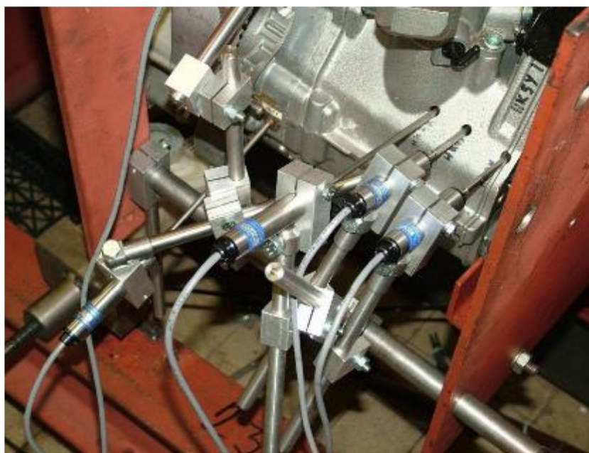
Figure 4-1: Example of the shaft deformation measurement under certain loading conditions in the laboratory of the TU of Ostrava
