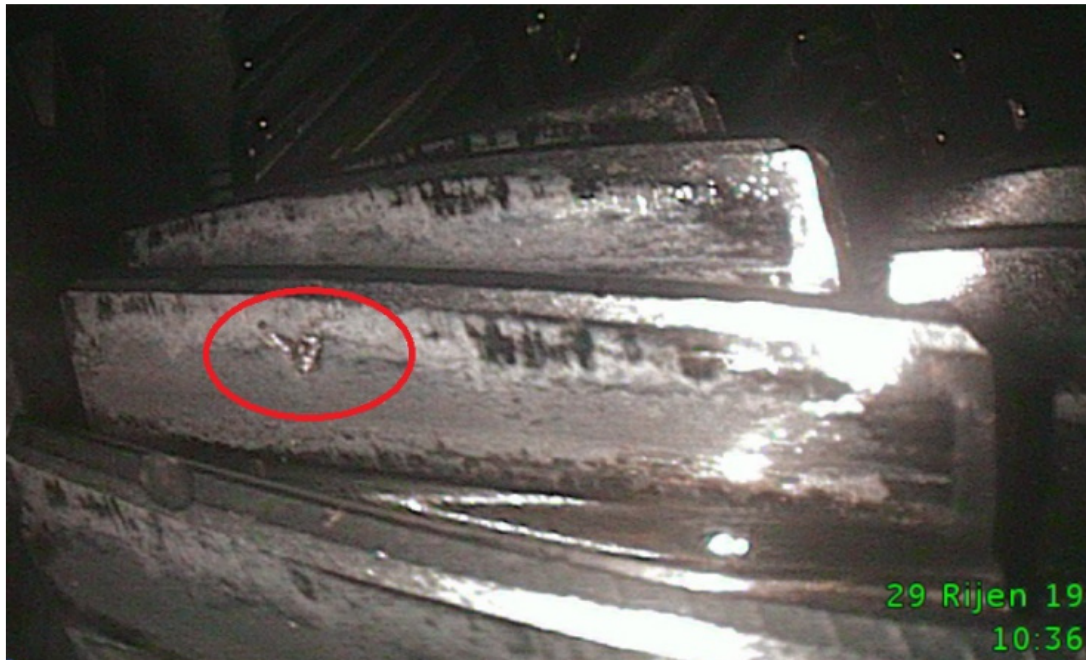
Figure 7-15: Pitting on PM HIP:ed gearwheel (3 rd speed pinion) – gearset 2 - after 100 hours
