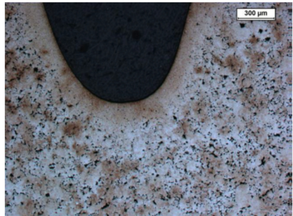
b) Large gear (z=48) – root etched
