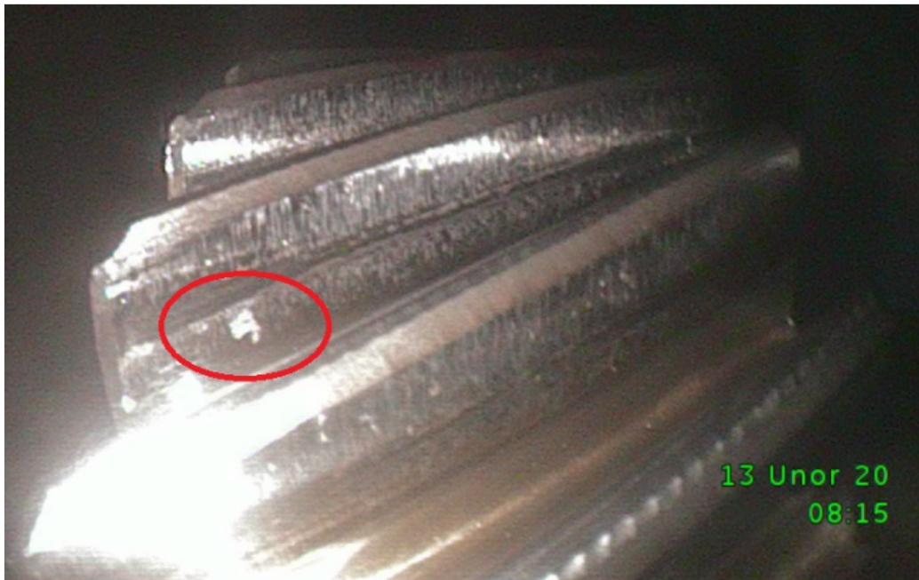
Figure 7-21: Pitting on PM HIP:ed gearwheel (6 th speed) – gearset 1 - after 85 hours
