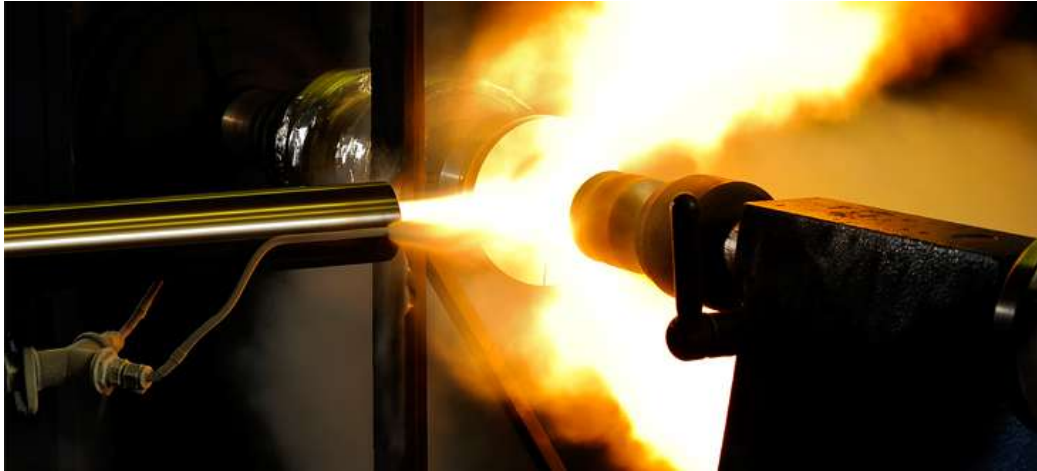
Figure 2.7: Detonation gun spray process. Image courtesy of Praxair Surface Technologies, USA.
