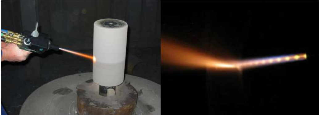
Figure 2.8: High velocity oxy-fuel spray process (HVOF). Hand-held torch (left) and illustration of Mach diamonds from the supersonic flow of gases (right). Images courtesy of Avweld, Australia.
