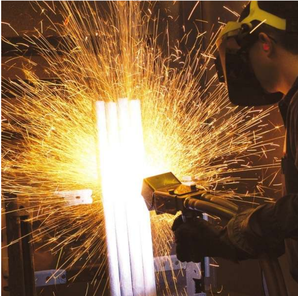
Figure 2.6: Wire arc spray process. Image courtesy of Office of Technology Commercialization, University of Minnesota, USA.
