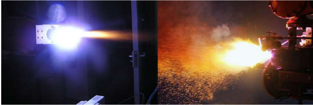
Figure 2.9: Plasma spray processes. Standard DC gas-stabilized torch (illustrated using SG-100 torch, Praxair Surface Technologies, USA, left) and hybrid water-stabilized plasma (WSP-H500, Institute of Plasma Physics, The Czech Academy of Sciences, Czech Republic, right). Own research.
