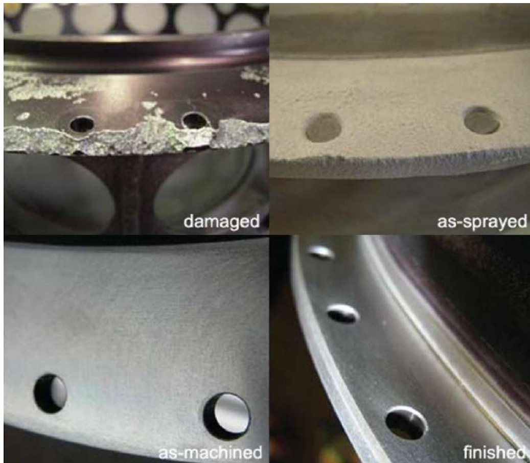
Figure 2.15: Restoration of worn or damaged components by cold spray. The speed of cold sprayed coatings build-up and their ease of machining, mechanical strength, and superior adhesion offers significant economical advantage over other restoration processes [73].
