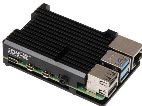
(a) : RasPi enclosed within the heatsink[18]
