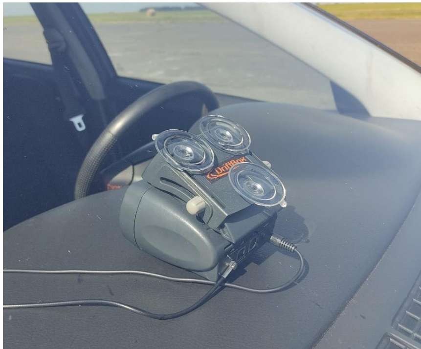
Figure 32 - RaceLogic DriftBox placement
