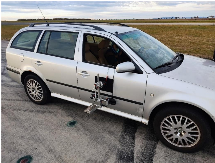
Figure 31 - Skoda Octavia with measuring devices
