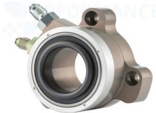
Figure 45 Clutch Release Bearing from SACHS used in Corbellati Missile
