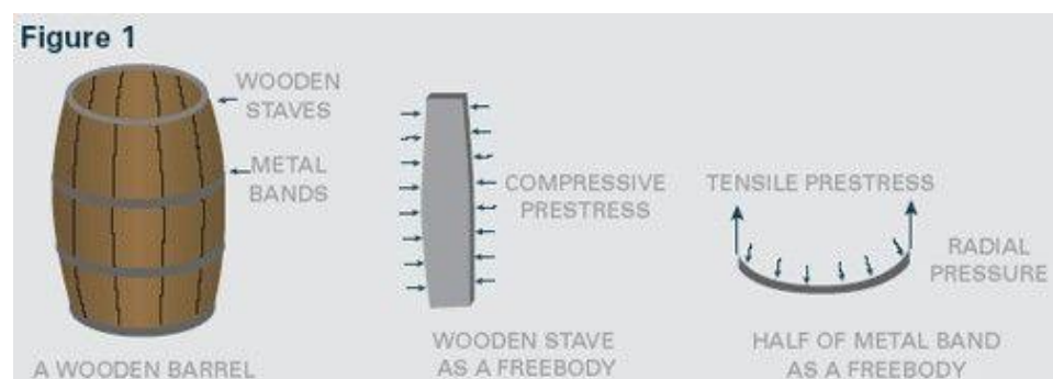
Figure 1: Introductory principle of prestressing
