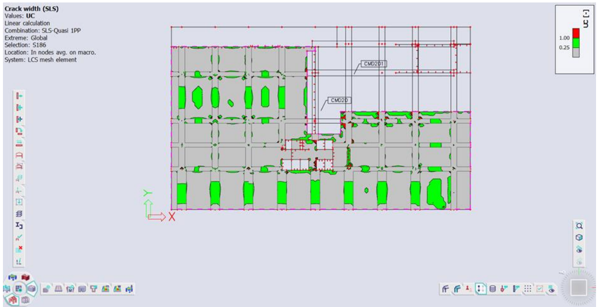
Figure 97: Display showing prestress crack width check for entire floor of 1PP due to SLS
