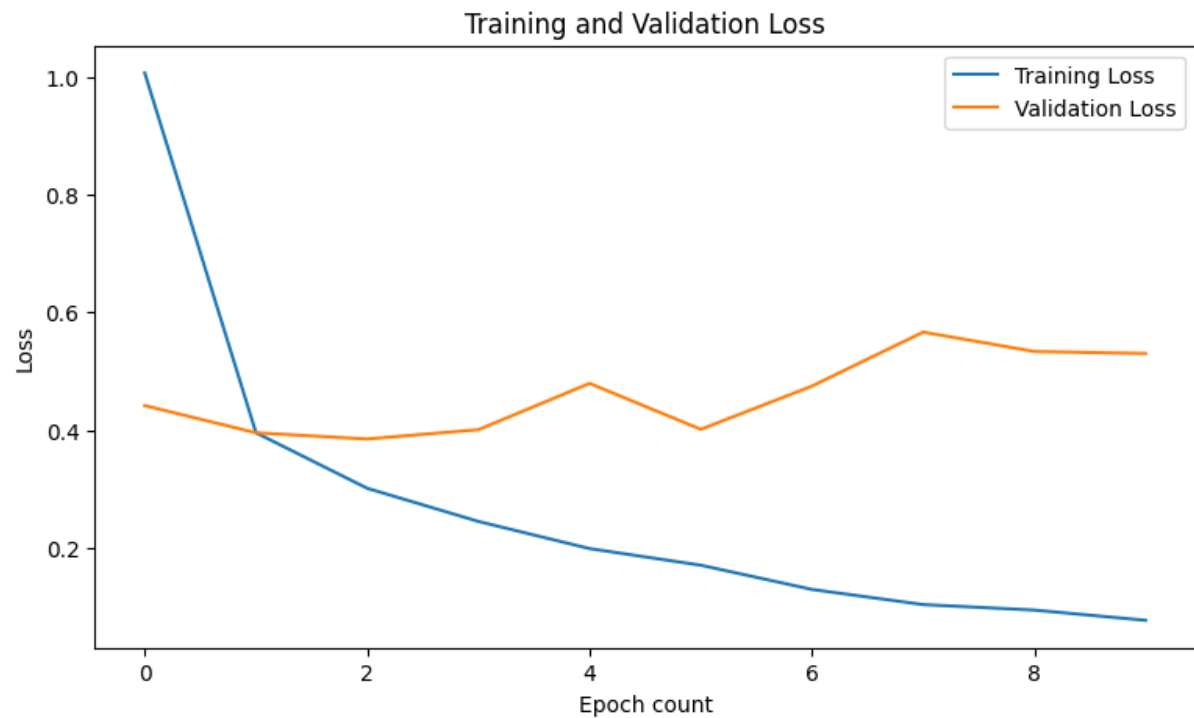
Figure 64: Loss of the training and validation set with the training/testing ratio of 80/20.
