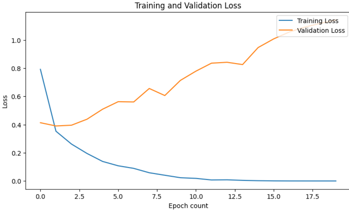
Figure 72: Loss of the training and validation set for track segment dataset size of 300.
