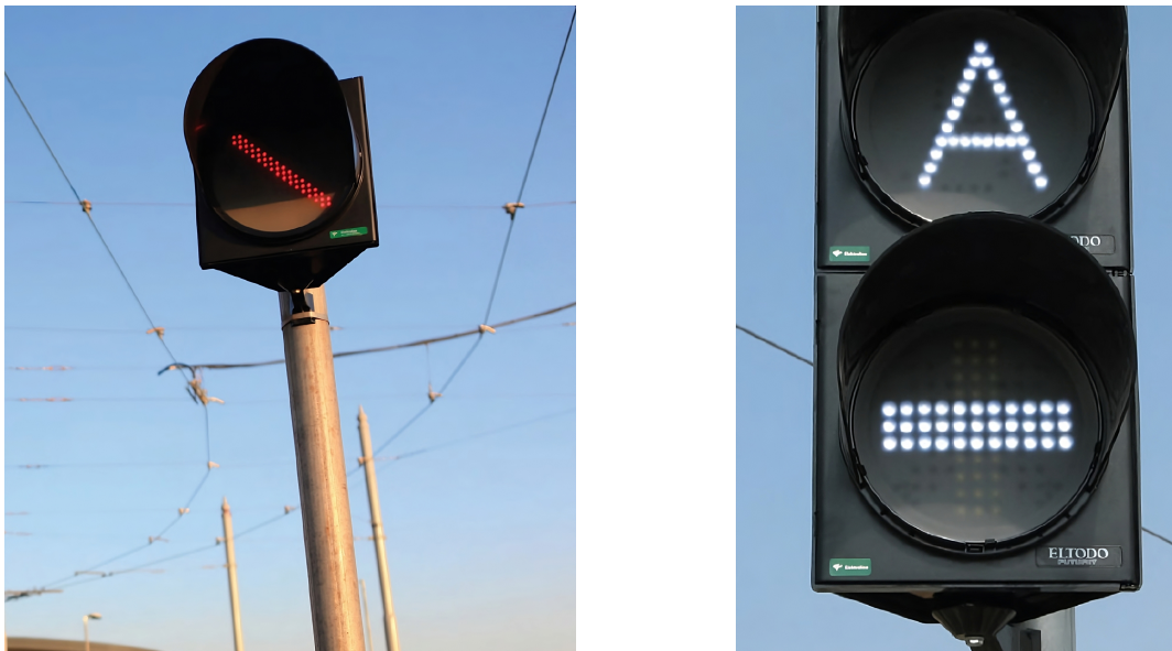
Figure 5: PPI signal lamp (left) and SG signal lamp (right) [2]
