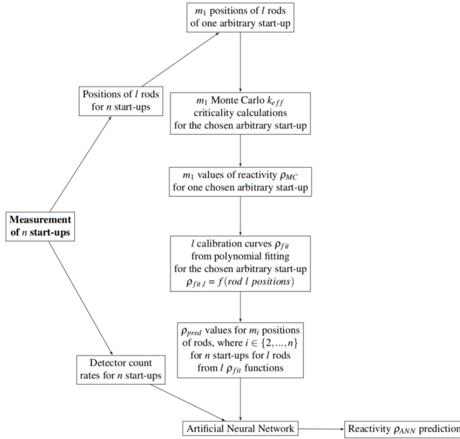
Figure 3.1: Scheme of the workflow to train and test an ANN to predict reactivity. Where l is the number of control rods, n is the number of collected start-ups and m_i is the number of positions of control rods for the i -th start-up.
