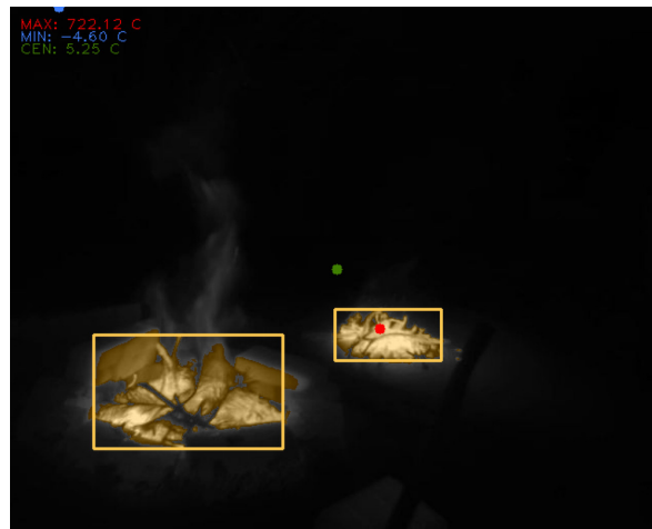
Figure 2.1: Thermal image with highlighted detected fires showing two separate fires and their detected bounding boxes.
