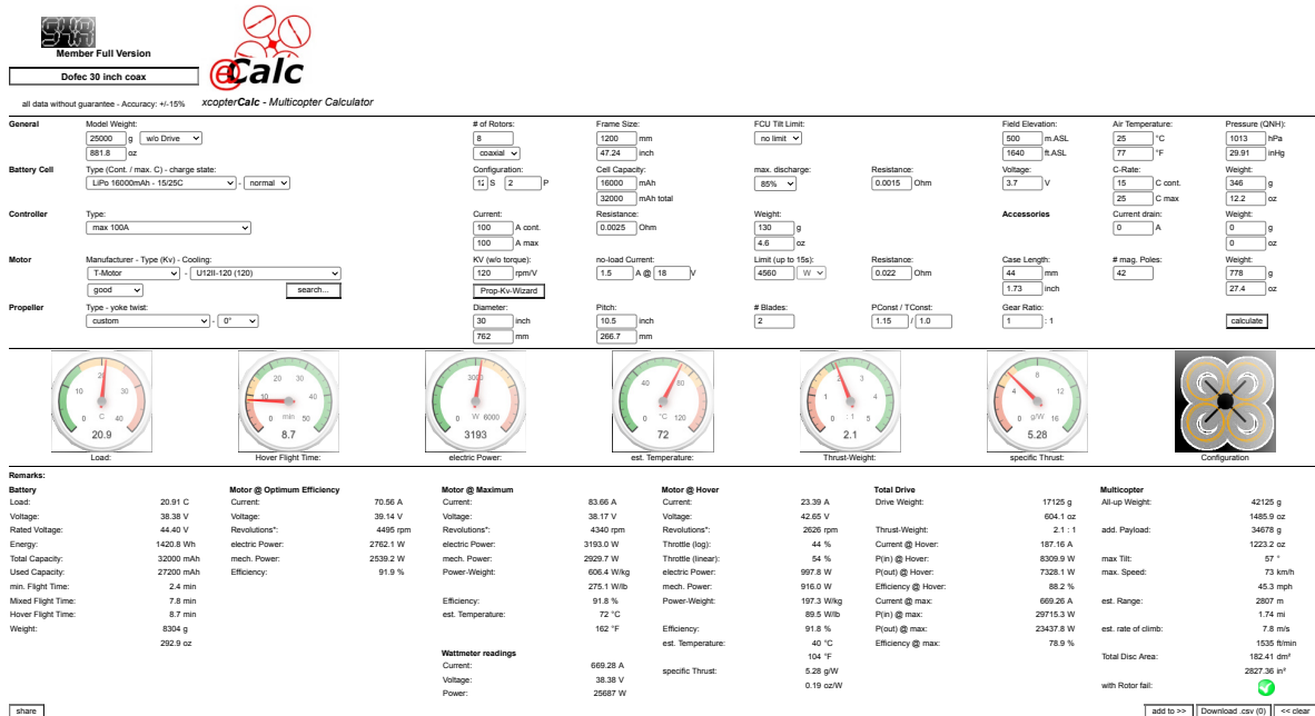
Figure 3.8: UAV design characteristic using the eCalc web tool [2].
