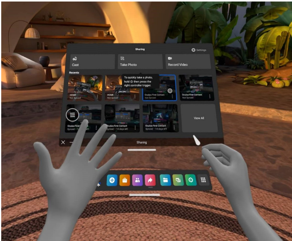
Figure 2.7: Quest 2 has in-built hand tracking, using its camera as input to track the hands. Gestures such as pinching, as shown in the image with the right hand, act as buttons.
