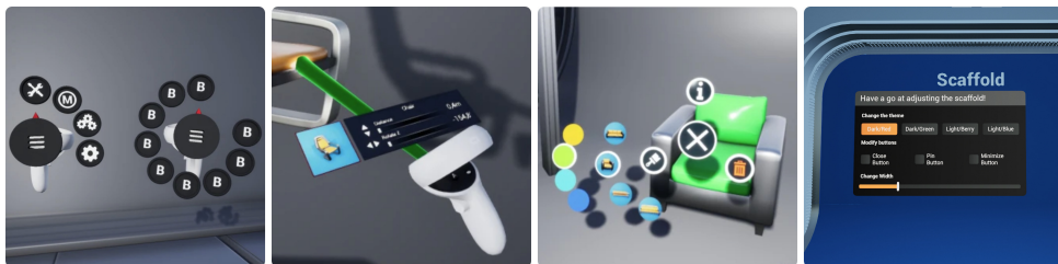
Figure 2.11: Examples of common VR interface elements. From left, radial menu, controller attached menu, object attached menu, floating window. (images from Advanced Framework - VR [20])
